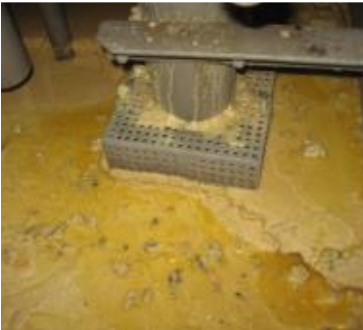
A ship's cargo hold bilge significantly clogged by melted cocoa butter
