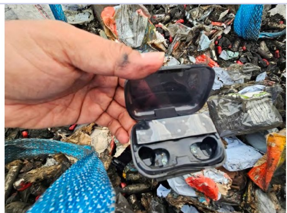
20. The view of TWS (True Wireless Stereo) one of the cargo found damaged and melted.
