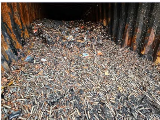
11. The view of the small batteries type 18650 in damaged condition was scattered in the damaged Container No. EGHU 8316805.
